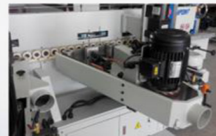
成型三角环带砂 Profile belt sanding unit Motor : 2HP Sanding belt size : 4" x 98" / 84" Vibration power : 25w x 1/36
