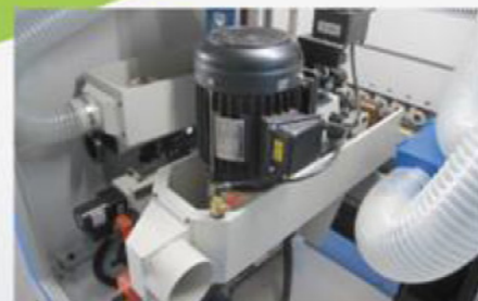
平面三角环带砂 Belt sanding unit Motor : 2HP Sanding belt size : 4" x 60" Vibration power : 25w x 1/36
