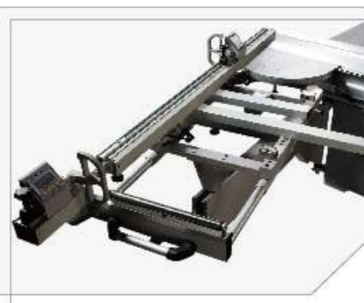
+ 47° ~ - 47° Tilting Cross-cut Carriage With Digital Display And Quick Position At 22.5° And Each 5°
