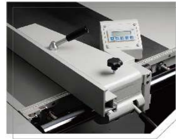
Digital Display On The Rip Fence
