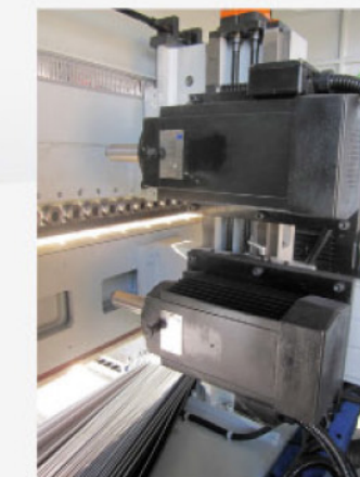
Top and bottom milling unit 5HP(special 7.5HP) Spindle speed:3600/7200 rpm (60/120HZ) Spindle dimension:Ø40 x 82 mm (L)
