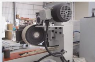
GV7 Grooving unit Cutting groove on the work piece. Motor power 3 HP run at 3000 R.P.M Saw blade : 255*25.4*3.0*80T Spindle dia. : Ø25.4*82 mm(L)
