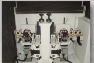
PM1 : Profile moulding unit PM(left hand) / PM2(right hand) Apply moulding on panel edge or lipping. Standard with H.F. motors. Spindle tiltable : 0°~180° Cutter : 80 x 20 MM / 120 x 30MM Speed : 12000 R.P.M. Motor : 5 HP Space required : 570 MM
