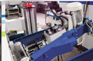
PS5 : Profile sanding unit PS5(left hand) / PS6 (right hand) Apply sanding on profile edge. Spindle tiltable : -15°~1+105° Belt size : 4" x 78" / 98" Belt speed : 630 MM Motors : 2 HP Space required : 750 MM
