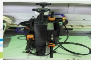
SC1 : Scrapping unit Apply for scrapping top and bottom corners of PVC / ABS. Spindle fixed at 45° Scrapping blade : Subject to order with radius required. Space required : 400 MM
