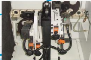
ET2 : Tilting edge trimming unit Apply for fine trimming of top and bottom edge as "chamfering". Spindle tiltable : 0°~35° Cutters : 80 x 20 MM / 100 x 20 MM Speed : 12000 R.P.M. Motors : 0.75 HP x 2 / 2.5 HP x 2 Space required : 645 MM
