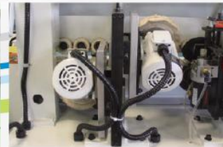
BS1 : Brushing unit Apply the finest surfacing process on top and bottom edge. Spindle tiltable : 0°~45° Brushing wheel : 180 x 25 MM Speed : 1750R.P.M Motors : 0.5 HP x 2 Space required : 510 MM
