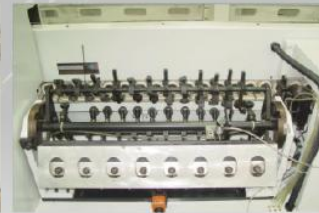
SP2 : Rotary side pressure unit (1) Vertical pressure rollers for pressing straight edge. (2) Profile pressure rollers for pressing softforming edge. Space required : 870 MM
