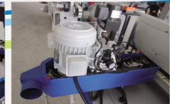
PS7 : Belt sanding unit Sanding Motor: 2HP Sanding belt size: 4" x 60" Vibration power: 25w x 1/36
