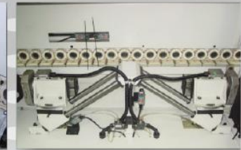
EC1 : End cutting unit Apply for cutting front & rear edge by (2) independent motors. Spindle swivable : 0°~45° Sawblade : 150 x 200 MM Speed : 12000 R.P.M. Motors : 0.67 HP x 2 Space required : 1155 MM
