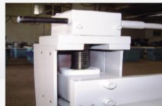
The top pressure beam equipped with ball screw transmission
