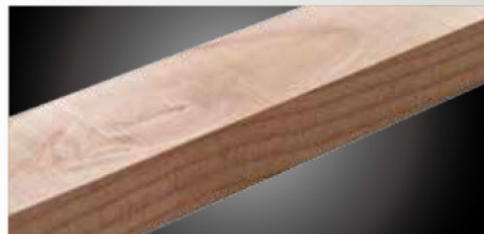
Without jointer device, the timber have clear cutter mark.
