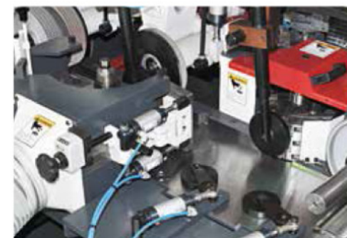
Jointer Device Jointer device allows the cutter service time to be extended. It also ensures no cutting marks exist on the machining surfaces, while creating extra fine surface finishes.
