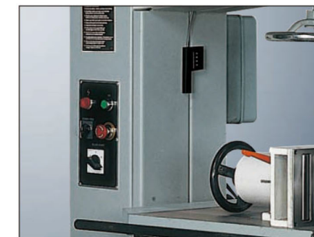
ELECTRICAL CONTROL PANEL The electrical control switches are centralized on a control panel for operation convenience. The blade start is controlled by a Y-starting switch for safe and smooth starting of the blade.
