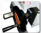
手動進退調整輪 Manual forward/ backward control handwheel
